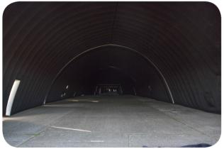
Inflatable tunnel for testing ADAS in complete darkness.
