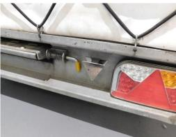
**Left image:** Impact Protection Vehicle (IPV) after being struck by an HGV (stopped past IPV after striking). **Right Image:** RadViz fitted to a vehicle to improve its likelihood of detection by Automatic Emergency Braking Systems (AEBS) on lorries and cars by increasing its radar signature.
